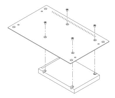
Step1. Fix HDD using the 4 screws in the Accessory Kit.
