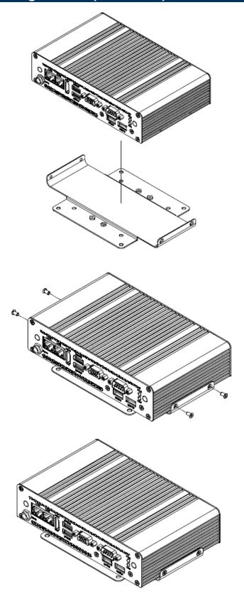
**Step1.** Insert and fasten 4 screws on each side of the system to secure Mounting bracket.
