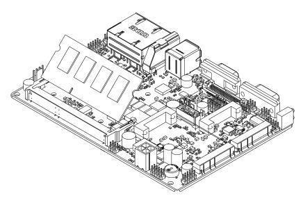
**Step2.** Properly install the memory module and press until properly seated.
